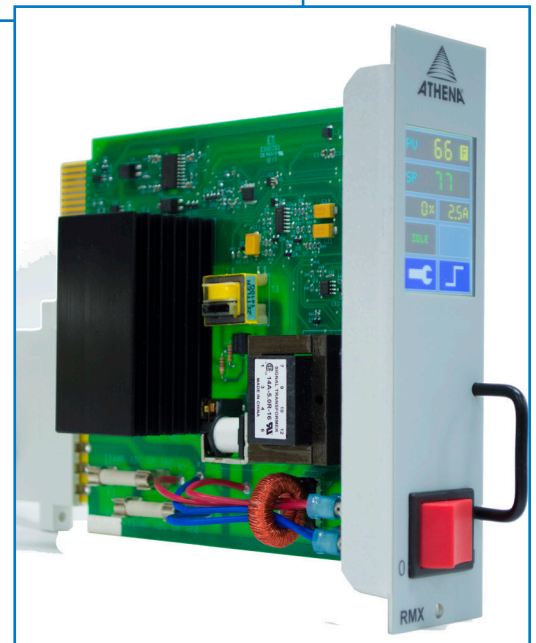
Fig 1. RMX Modular Controller showing single zone temperature control from touchscreen.
