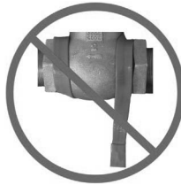
A.) Incorrect Installation: Heating tape hanging free from the surface
